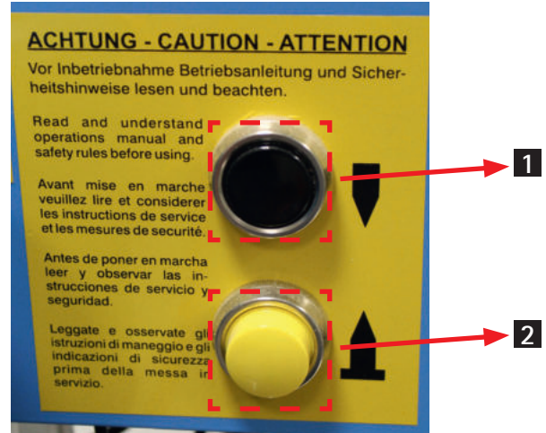
Fig. 37: Manually operated valve and momentary switch
