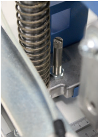
Fig. 30: Drill depth stop with hexagon head screw
