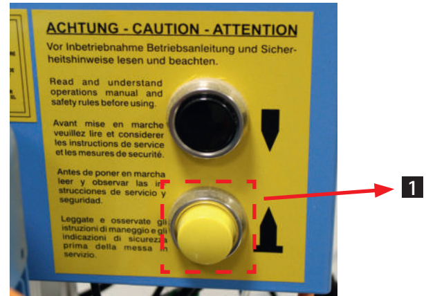
Fig. 27: Yellow button: Releasing the hold-down clamps
