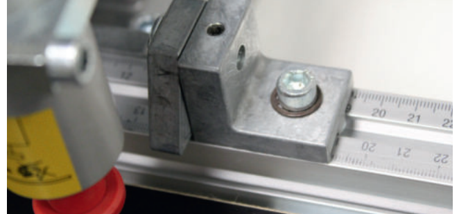
Fig. 32: Pendulum stop with hexagon socket screw
