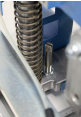
Fig. 22: Setting drilling depth
