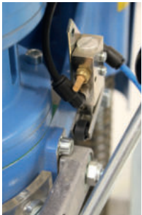
Fig. 20: Swivel unit with sensor roller
