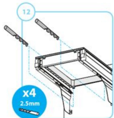
Center tray, mark and drill holes
