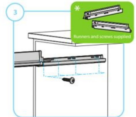
Mount runners as per manufacturers instructions (runners and screws not supplied)
